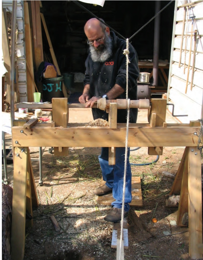
Figure 8: The author turning a bowl on a pole lathe, 2003. Photograph: David Harrison.
