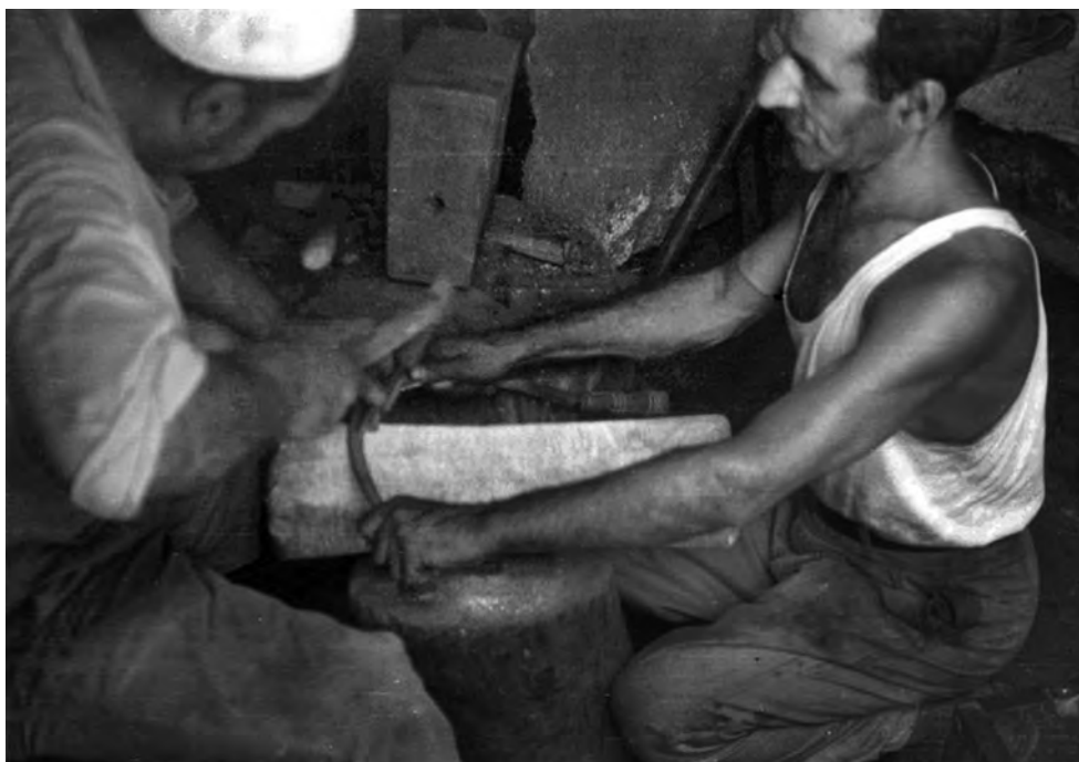
Figure 5: Blacksmiths of the Zoabi family in Nazareth serrating a sickle (Avitsur archive).
