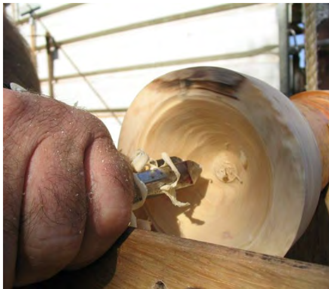
Figure 9: Turning the interior of the bowl, 2003. Photograph: David Harrison.
