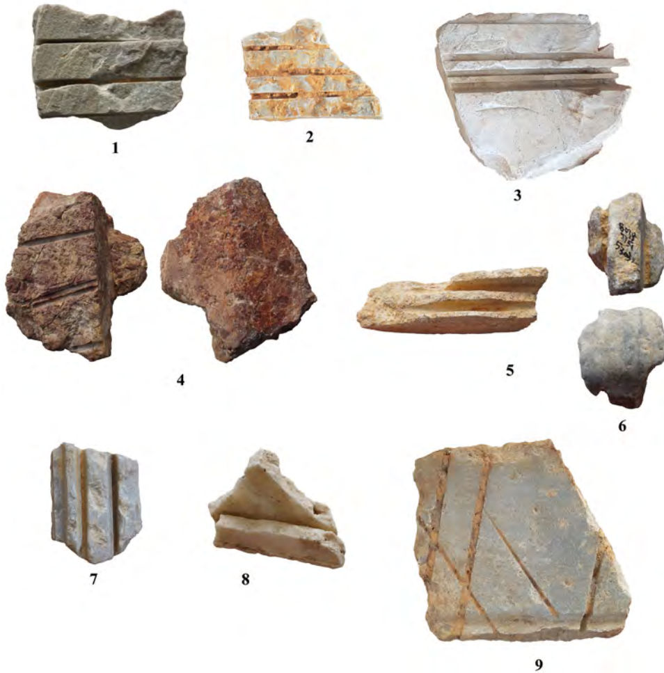
Figure 2: Sawing leftovers: 1–6, 9 from the area of the Octagonal Church complex; 7–8 from near the complex identified as Antoninus Pius Thermae. 1, 2, 6, 7, 9 white and grayish marbles; 3 bitumen; 4 conglomerate; 5 limestone; 8 calcite-alabaster.
