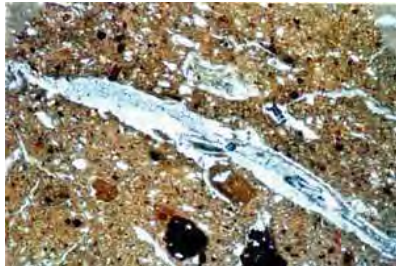
Fig. 4.1. Elongated pores (a larger one in the center) from burnt out straw in calcareous silty clay matrix incorporating quartz and opaque minerals, as well as few grog (center below) and rounded micritic limestone (upper left corner). Width of field 2.4 mm. Plain polarized light (PPL).
